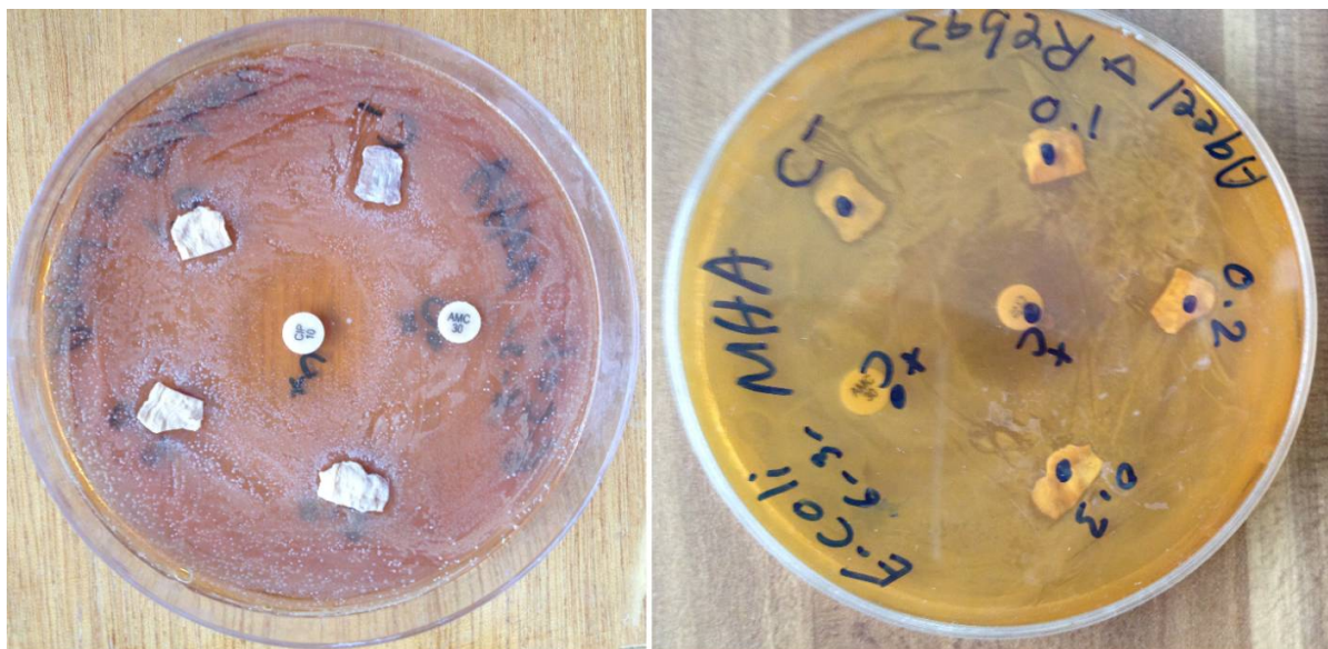
Fig. 3: Inhibition effect to Zn/nylon 6,10 on Escherichia coli bacteria
